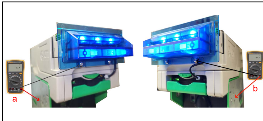
Figure 4 Resistance Measurements (Left/Right Sides of iVIZION Chassis Frame)
